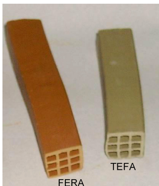
Fig. 1. Monoliths extruded in the laboratory with FERA and TEFA clays.
